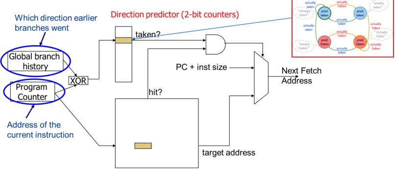
Cache of Target Addresses (BTB: Branch Target Buffer)
